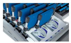
Micro-motor controllers precisely align each print head – creating a seamless image across the corrugated sheet to deliver the high print quality results.
